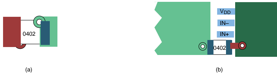
Figure 13. Typical Decoupling Capacitor Layouts
